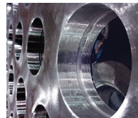
Sure-Lock ring grooves make 40% stronger joints
